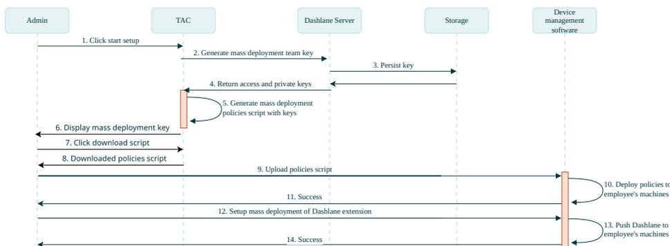
Figure 7: Credential Risk Detection Mass Deployment process
